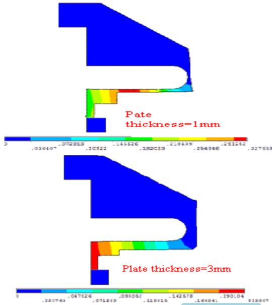
Fig.7: Deflections values of various plate thicknesses
