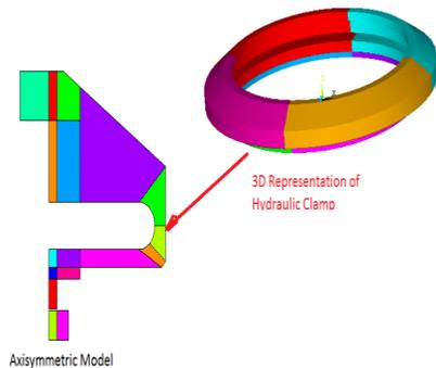
Fig.2: Ansys model of Hydraulic clamp
