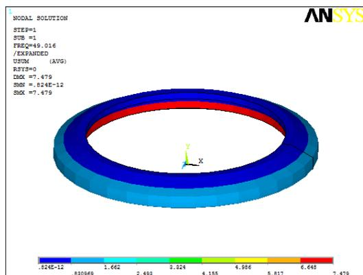
**Fig.10: Mode shape for first fundamental frequency 49.016Hz**
