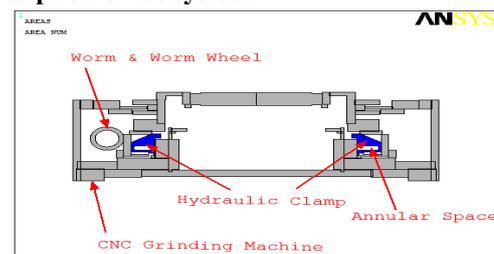
Fig.1: Hydraulic clamping system.
