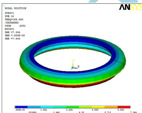
**Fig.11: Mode shape for second frequency 169.7 Hz**
