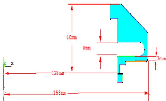
Fig.3: Dimensional plot of the Hydraulic clamp.
