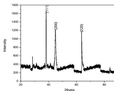
Figure4: X-ray diffraction patterns of synthesized Pt NPs.
