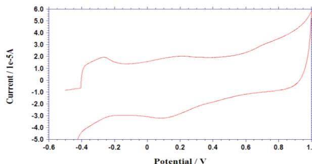
Figure 8: Cyclic voltammograms of platinum nanoparticles
