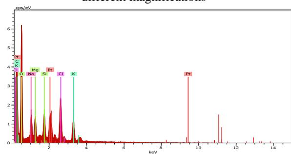
Figure 6. EDX spectrum of platinum NPs capped with Croton Caudatus Geisel leaf extract
