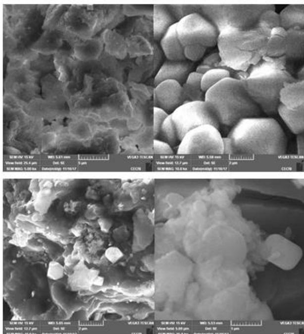
Figure 5: SEM images of platinum nano particles at different magnifications
