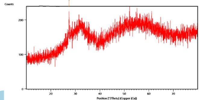
Fig:1 XRD pattern of ZrO<sub>2</sub> nanoparticle
