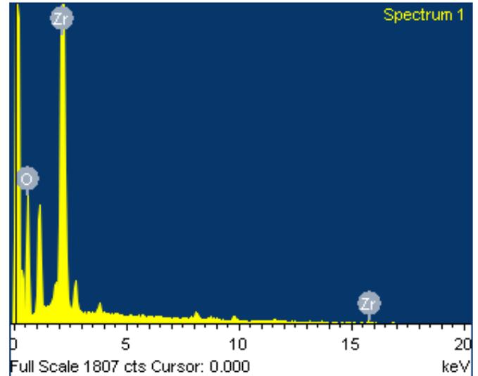
Fig:5 EDAX Spectrum of nano ZrO<sub>2</sub> mixed oxide
