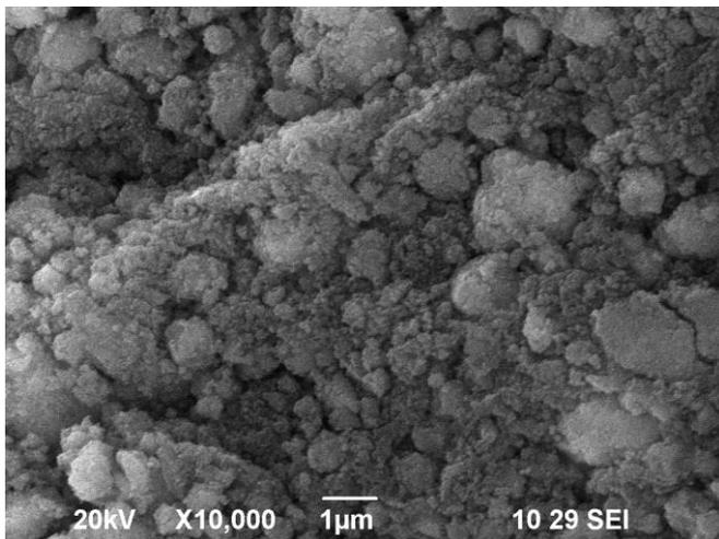
Fig:4 SEM image of nano MoO<sub>3</sub>-ZrO<sub>2</sub> oxide
