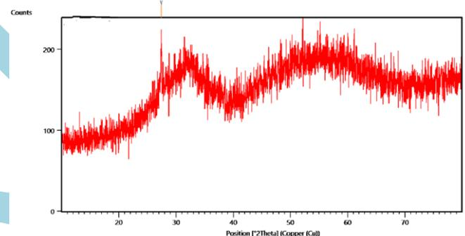
Fig:2 XRD pattern of MoO<sub>3</sub>- ZrO<sub>2</sub> nanoparticle
