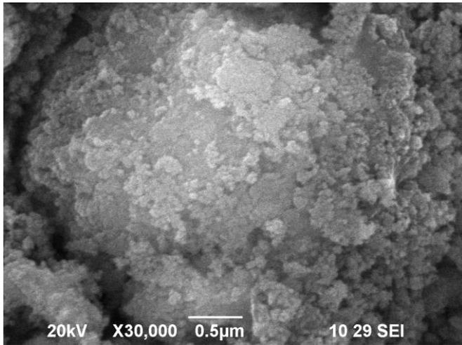
Fig:3 SEM image of nano ZrO<sub>2</sub> oxide
