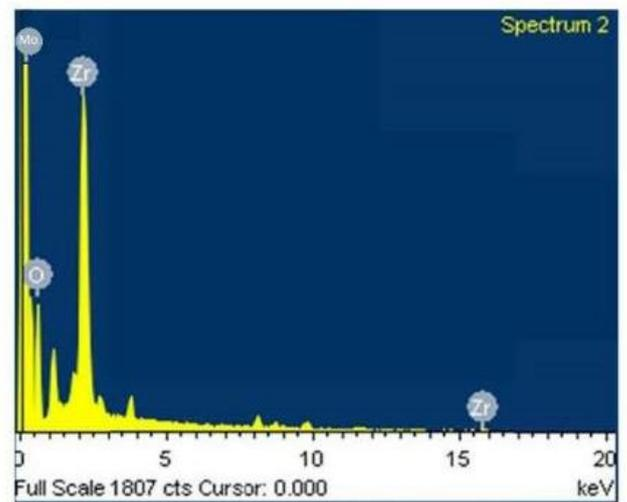
Fig:6 EDAX Spectrum of nano MoO<sub>3</sub>-ZrO<sub>2</sub> mixed oxide
