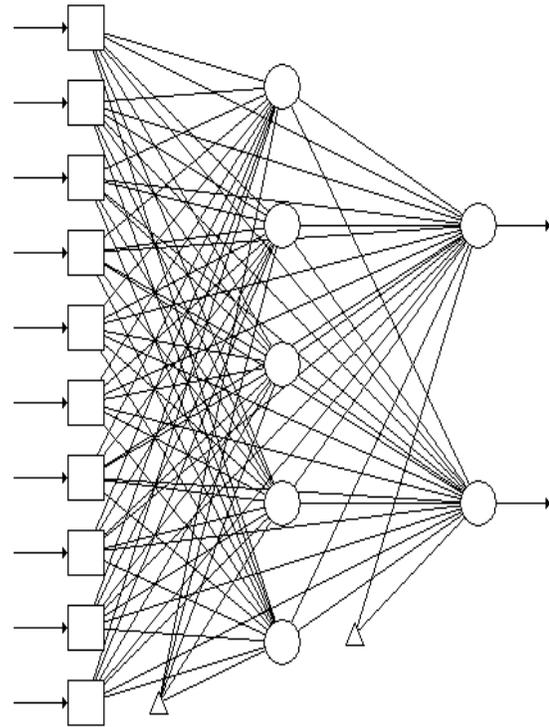
Fig.3 Topology for Feed-forward Neural Network used (10-5-2) in the study
