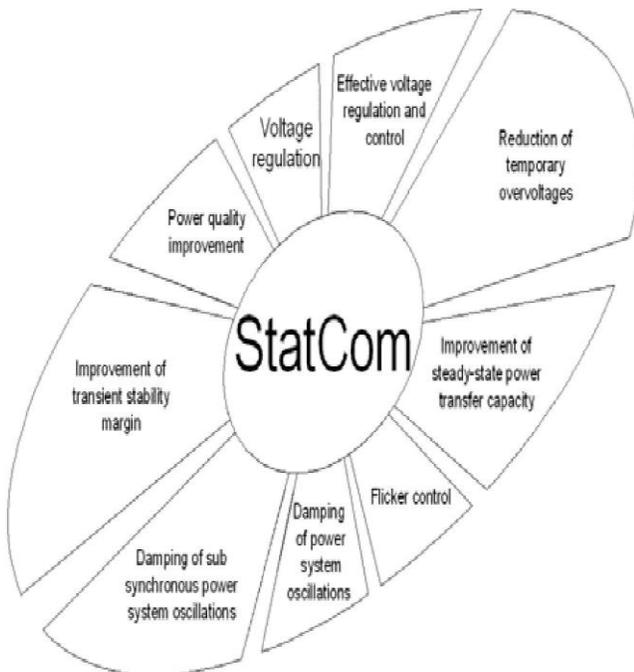
Figure-1 Typical applications of the STATCOM
