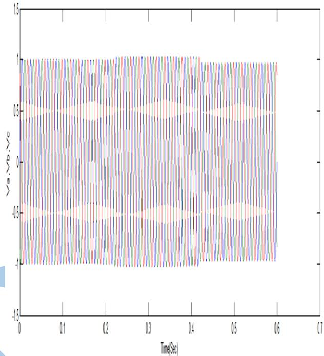
Figure-2. Three phase instantaneous voltages
