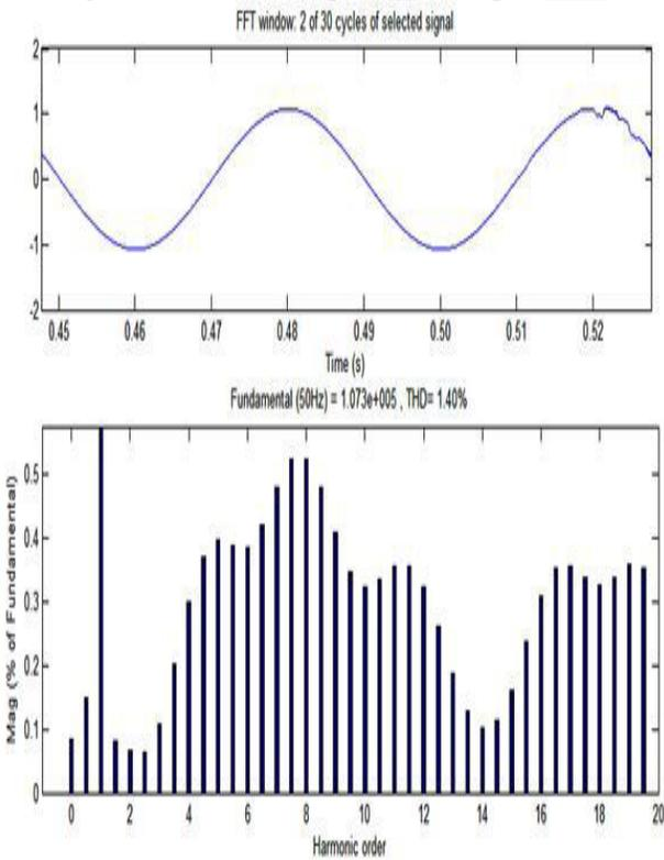
Figure-5 Voltage (Va) Spectrum in inductive mode
