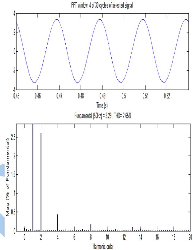
Figure-6. Current (Ia) Spectrum in Inductive mode
