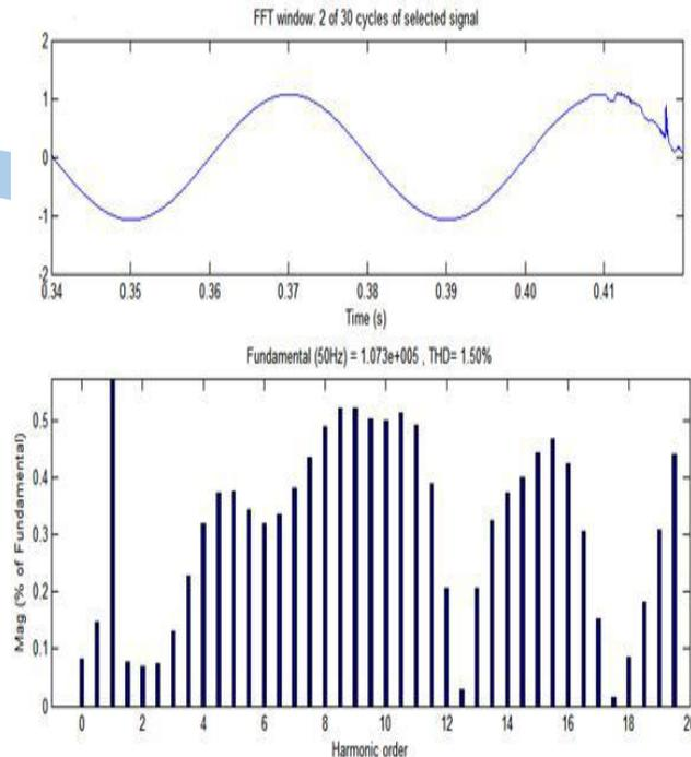
Figure-3. Voltage (Va) Spectrum in Capacitive mode
