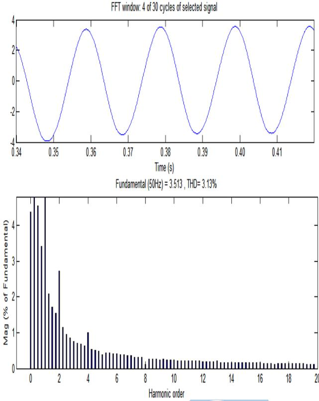
Figure-4 Current (Ia) Spectrum in Capacitive mode
