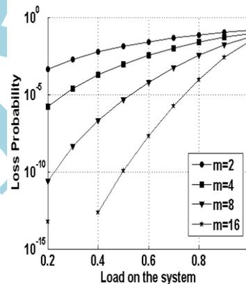
Fig. 3 Packet loss probability vs. load for different number of buffer module
