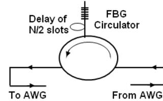
Fig. 2 Schematic of the buffer module
