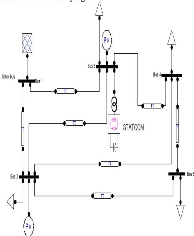
Figure 2. STATCOM-upgraded 5-bus system in PSAT
