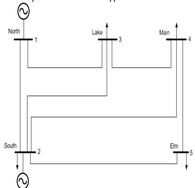
Figure 1. 5-bus Test System Source
