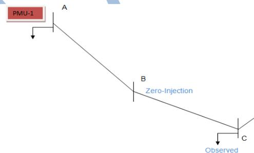
Fig.3.2 Zero-Injection Case
