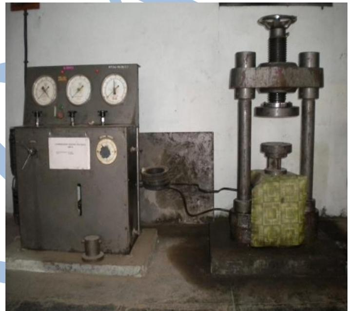
Figure 2 Picture showing Compression testing machine
