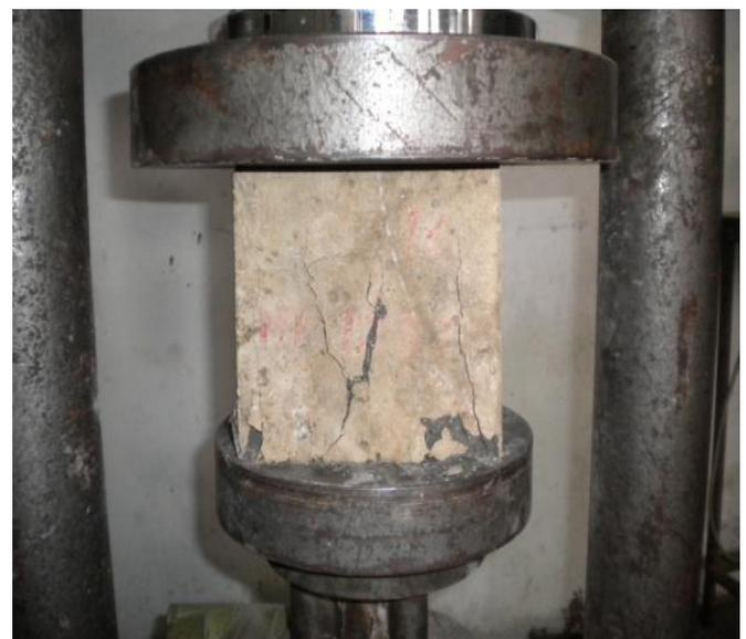
Figure 3 Picture showing Cube test
