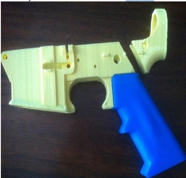
Fig [4]: Gun casted using 3D printing technology
