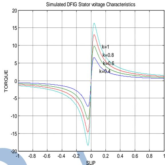
Fig. 3.2 Simulated DFIG Stator Voltage Characteristics
