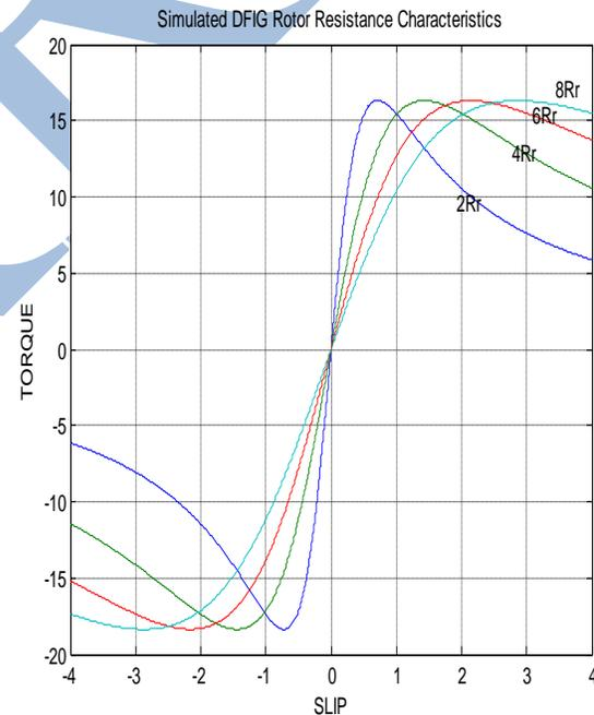
Fig. 3.3 Simulated DFIG Rotor Resistance Characteristics
