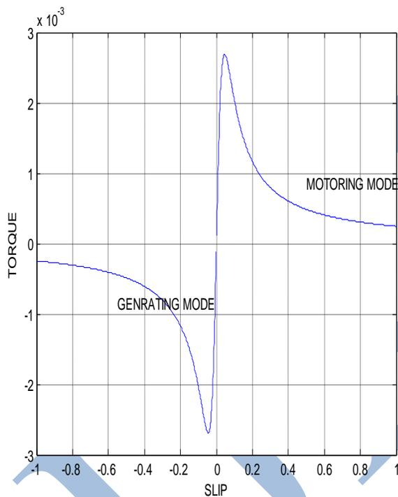
Fig.3.1 Torque speed characteristics of DFIG
