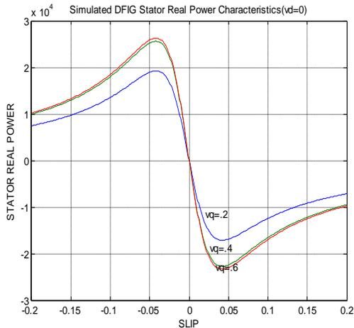
Fig.3.4 Simulated DFIG Stator Real Power Characteristics ( $V_d = 0$ )
