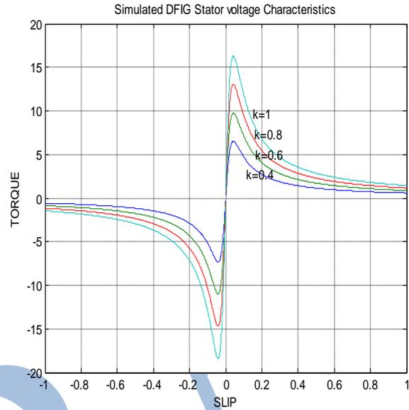
Fig. 3.2 Simulated DFIG Stator Voltage Characteristics
