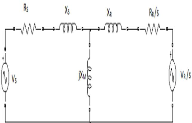
**Fig. 2.1 DFIG equivalent circuit with injected rotor voltage**
