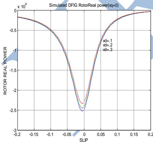
Fig.3.5 Simulated DFIG Rotor Real Power Characteristics ( $V_q = 0$ )
