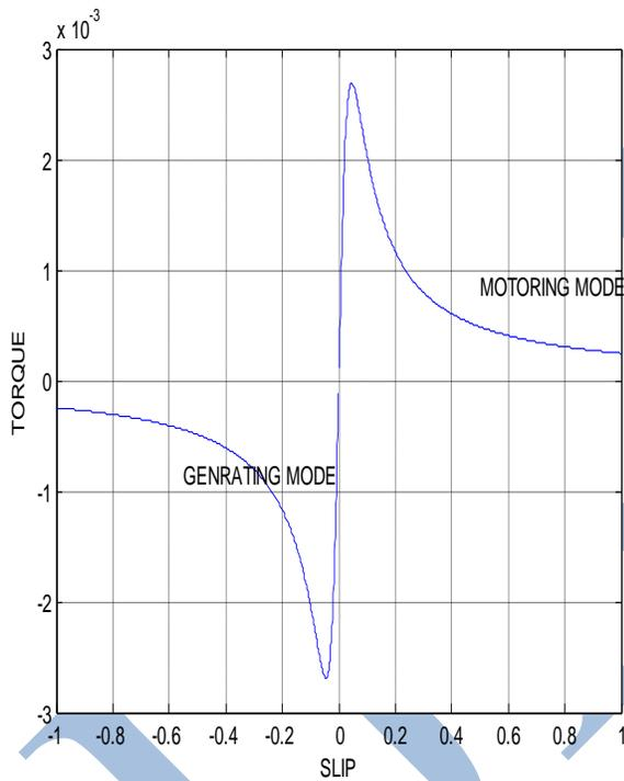
Fig.3.1 Torque speed characteristics of DFIG
