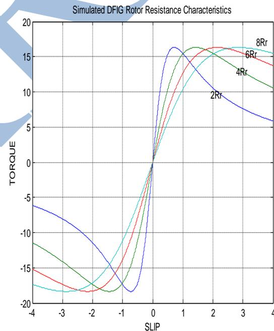
Fig. 3.3 Simulated DFIG Rotor Resistance Characteristics
