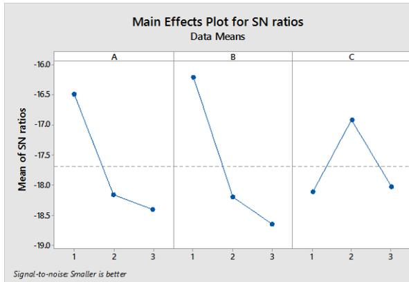
Fig 5.1 depicts the main effect plot for S/N ratio. It can be seen from Fig 5.1 that within the range of investigated input parameters, the optimal combination of the parameters surface roughness is A1B1 C2, i.e., at speed(A1) ,feed(B1) and amplitude(C2).
