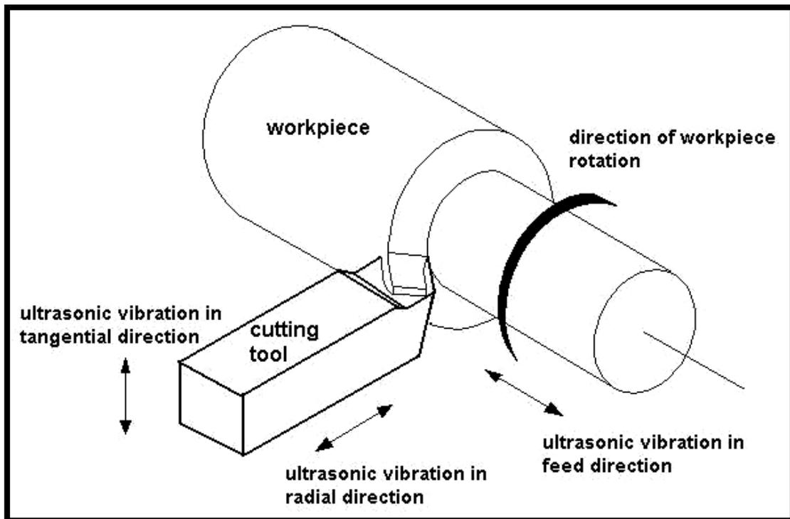
**Figure 1.1 Principal vibration directions during ultrasonically assisted turning**
