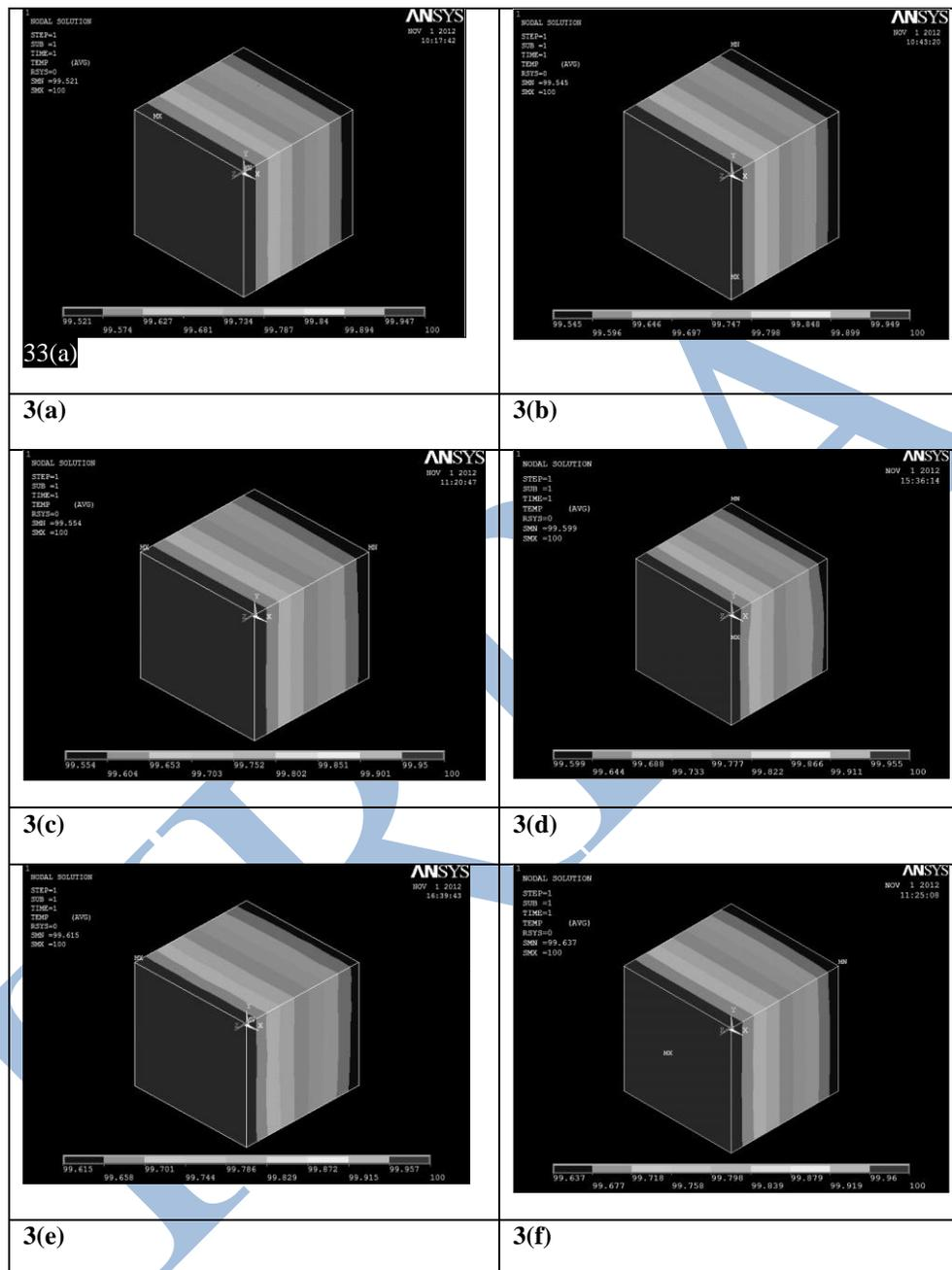
**Fig3**Temperature profiles for epoxy-BNcomposite with different filler concentrations 3(a) 1.5 vol%
