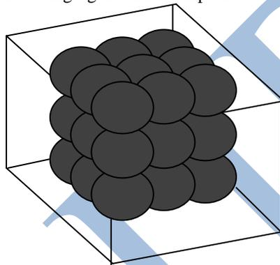
Fig. 1. Schematic diagram showing a typical arrangement of BN within the epoxy body
