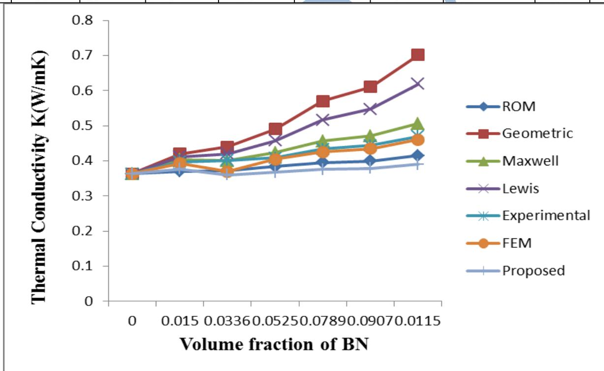
**Fig 4.Variation of effective thermal conductivity with BN content: Comparison of theoretical and measured values**
