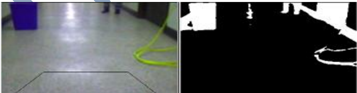
Figure 2.2: 1. Input color image with reference trapezoidal area 2. Binary obstacle output image
