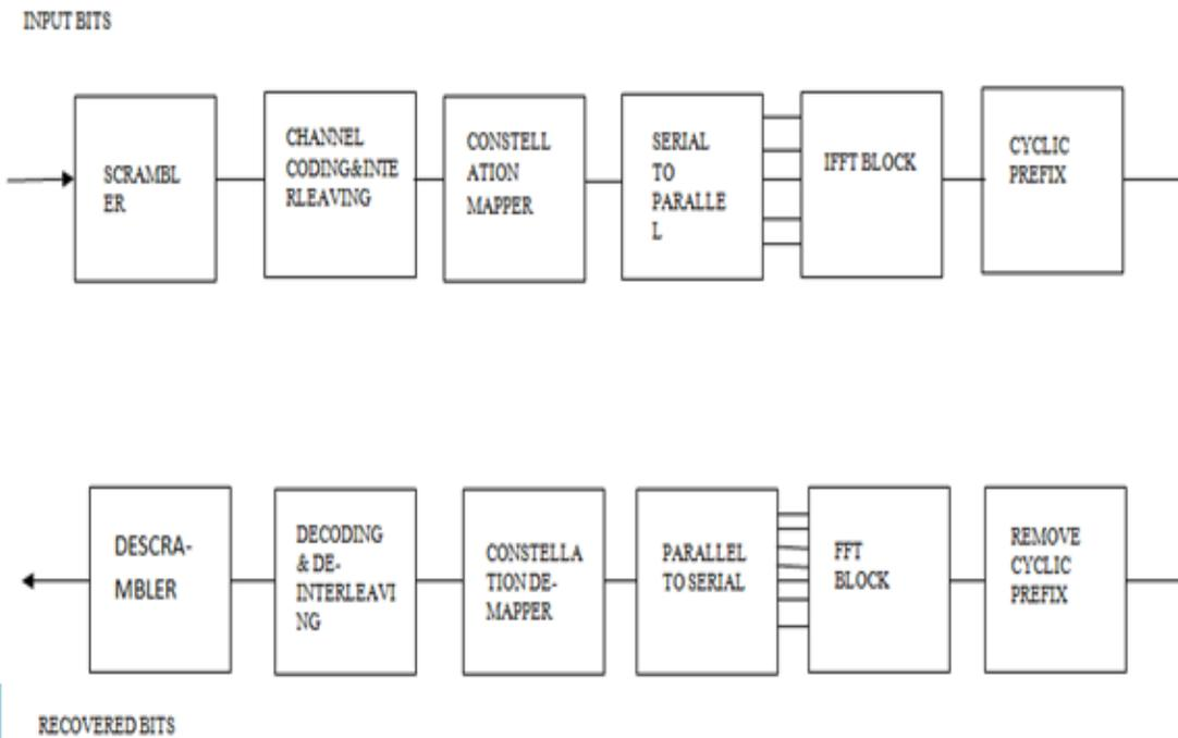
Fig2 Transceiver for 802 11 a
