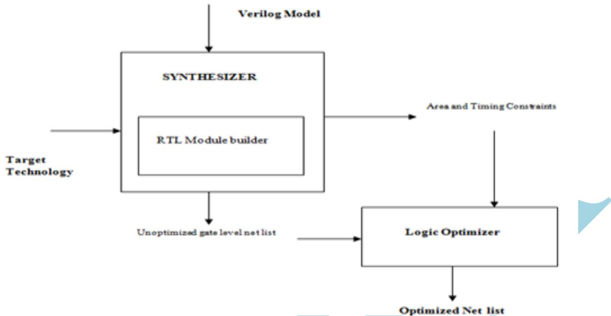
Figure 3 Synthesis Process in VERILOG
