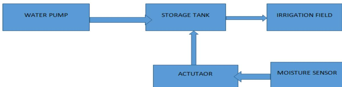
**Fig. 2: Block diagram of automatic irrigation module.**
