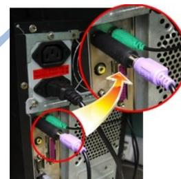
Figure 1. A hardware-based Keylogger
