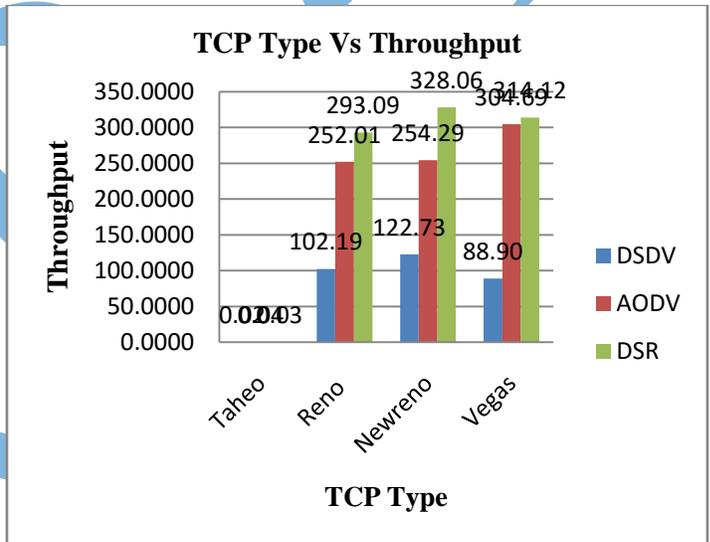
Graph 5.5: Throughput versus TCP types for different Protocols
