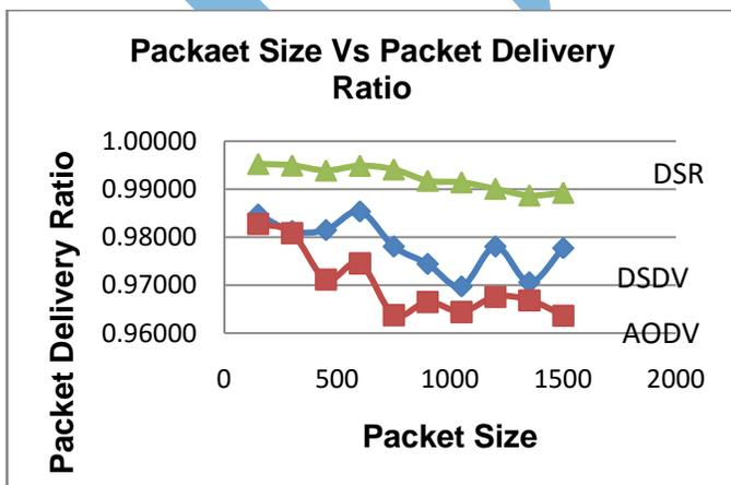
Graph 5.1: Packet Delivery Ratio versus Packets sizes for different Protocols
