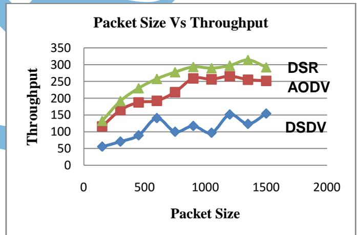
Graph 5.2: Throughput versus Packets sizes for different Protocols
