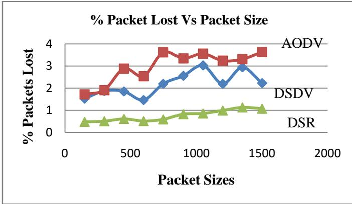
Graph 5.3: % Packets lost versus Packets sizes for different Protocols
