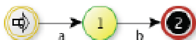
Figure 6: Automaton that represents the concatenation of two characters, 'a' & 'b' (ab) The alternation of a|b is constructed by adding a new state with a choice of first expression and another choice to second expression:
