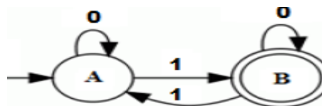
Figure 4: DFA for strings with an odd no of 1's.
