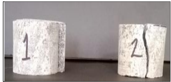
Fig.9 Failure mode of regular specimens (HP)
