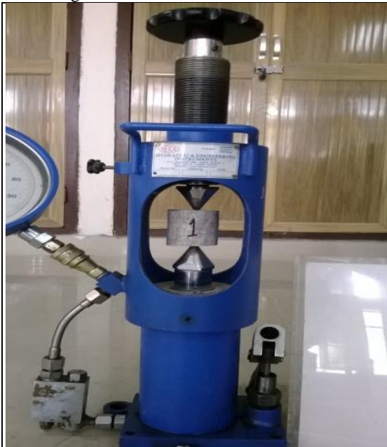
Fig.2 Point load test
