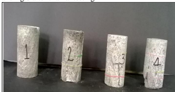
Fig.7 Failure mode of specimens (HP)
