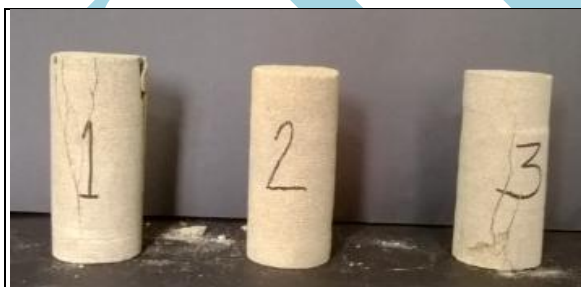
Fig.8 Failure mode of specimens (Jammu)
