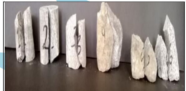
Fig.8 Failure mode of irregular specimens (HP)
