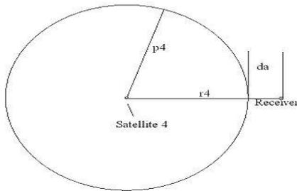
A satellite's position and distance from the receiver define a spherical surface, centred on the satellite. The position of the receiver is somewhere on this surface. Thus with four satellites, the indicated position of the GPS receiver is at or near the intersection of the surfaces of four spheres. (In the ideal case of no errors, the GPS receiver would be at a precise intersection of the four surfaces.)
