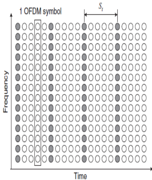
Figure 1.1 Block-type pilot arrangements.
