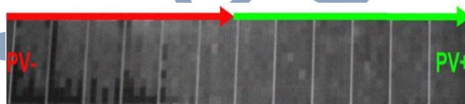
Figure 1: EL image of a floating PV string with degraded panels on the side with negative potential.[13]
