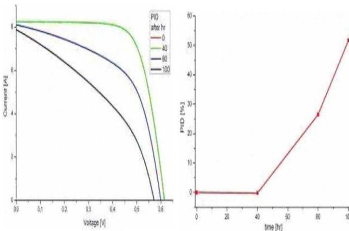
Figure 3: PID IV curve evolution (left) and corresponding power degradation (right). [14]
