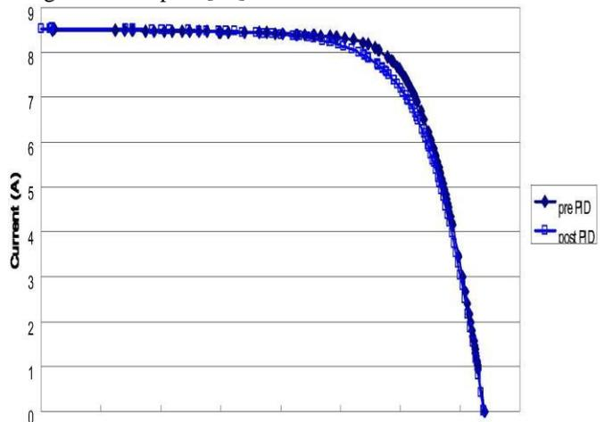
Figure 4: IV curve pre PID and post PID test. [14]
