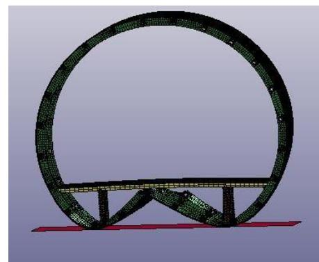
Figure 4 : LS-DYNA simulation (V= 10 m/s)
