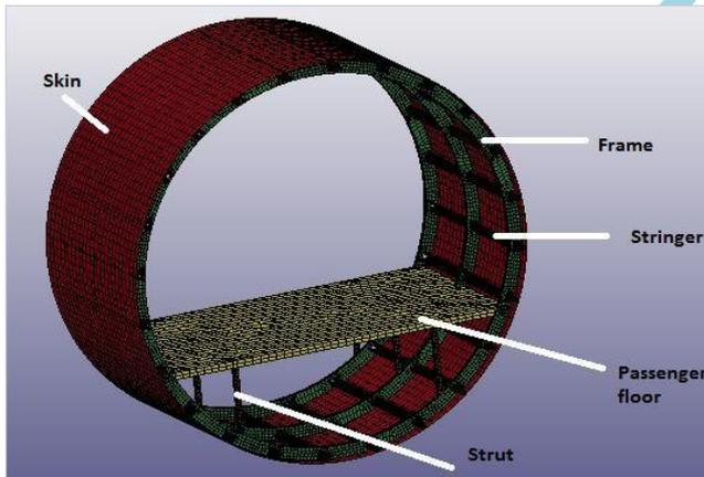
Figure 2 : Fuselage components
