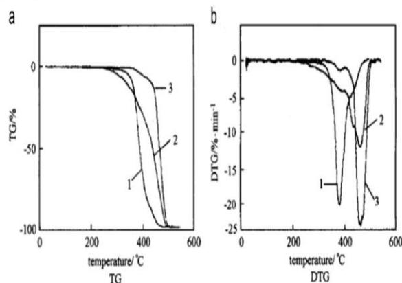
Figure 4.3 The pyrolysis TG and DTG plots of rubber materials.
