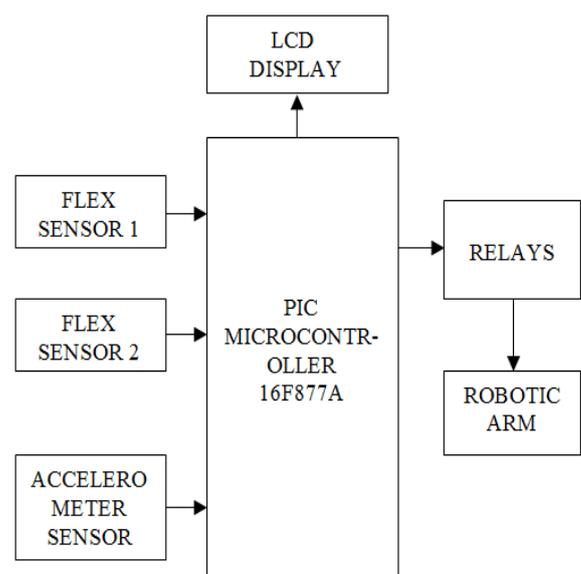
Fig1. Flex sensor based robotic arm using micro controller
