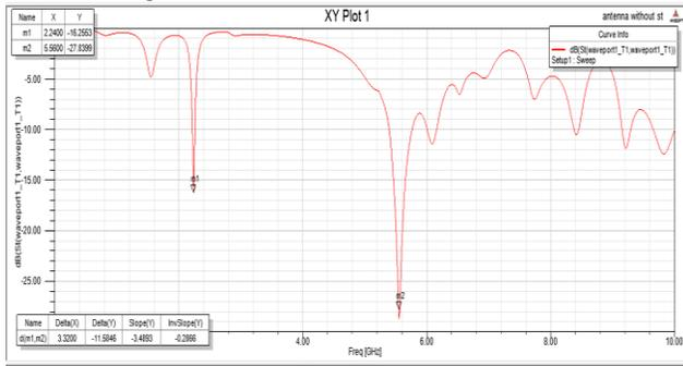
FIGURE 7.1.1 Return loss on normal human head.
