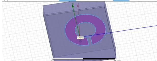
FIGURE 6.1.1 Ring shaped antenna
