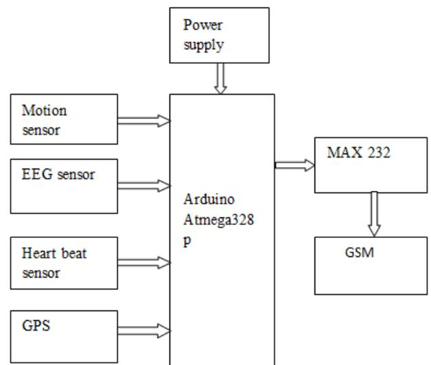
Arduino Uno is a microcontroller board based on the ATmega328 (datasheet). It has 14 digital input/output pins (of which 6 can be used as PWM outputs), 6 analog inputs, a 16 MHz ceramic resonator, a USB connection, a power jack, an ICSP header, and a reset button. It contains everything needed to support the microcontroller; simply connect it to a computer with a USB cable or power it with a AC-to-DC adapter or battery to get started.
