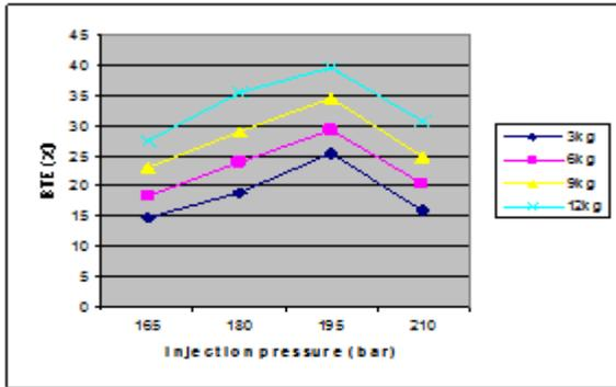
Fig 2. Variation of BTE with Injection pressure (B10)
