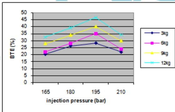
Fig 4. Variation of BTE with Injection Pressure (B30)
