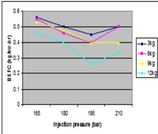
Fig 8. Variation of BSFC with Injection Pressure(B30)
