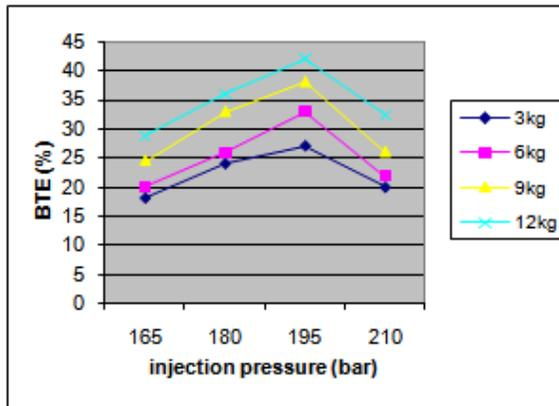
Fig 3. Variation of BTE with Injection Pressure (B20)
