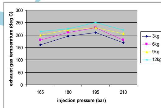
Fig 12. Variation of T<sub>exg</sub> with Injection Pressure (B30)
