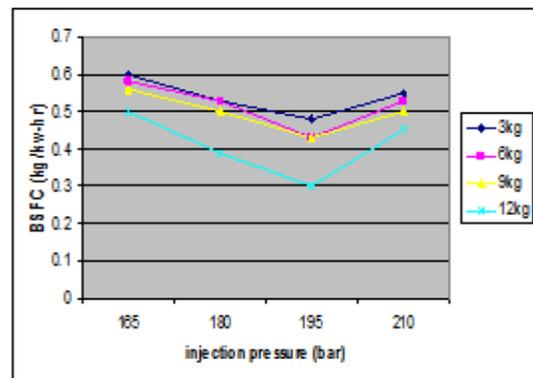
Fig 7. Variation of BSFC with Injection Pressure (B20)
