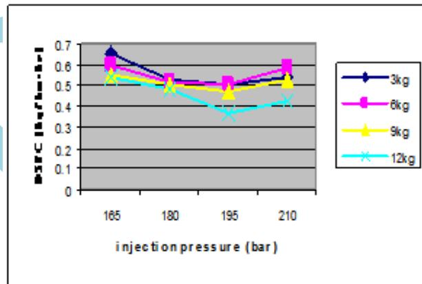
Fig 6. Variation of BSFC with Injection Pressure (B10)
