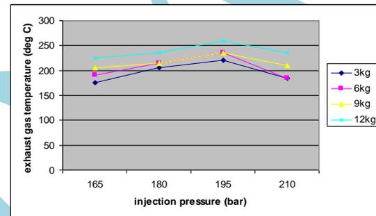
Fig 11. Variation of T<sub>exg</sub> with Injection Pressure (B20)
