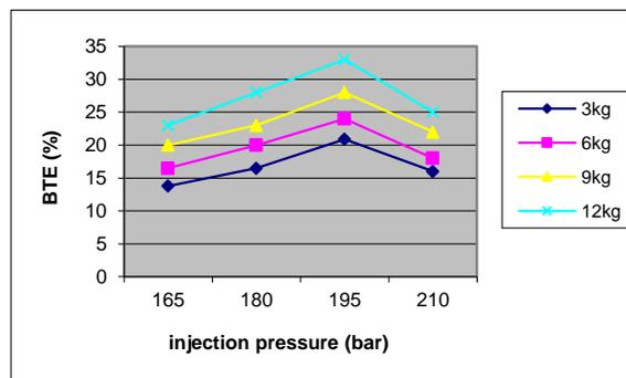
Fig 1. variation of BTE with Injection Pressure (100% diesel)
