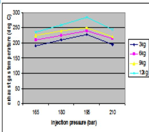
Fig 9. Variation of T<sub>exg</sub> with Injection pressure (pure diesel)
