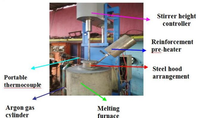
Figure 1 Modified stir casting machine
