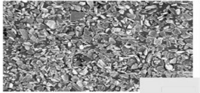
Figure 3 FESEM image of SiC<sub>p</sub>
