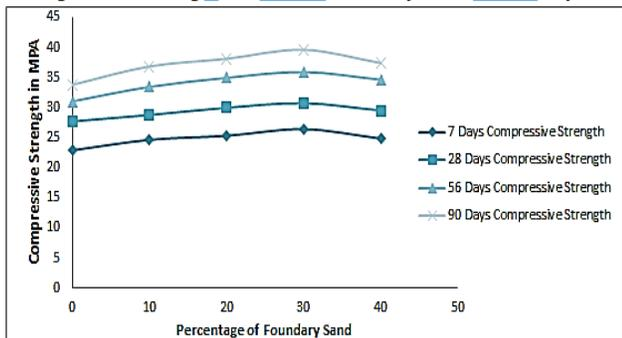
Figure-02. Compressive Strength and Percentage of Foundry Sand [4]
