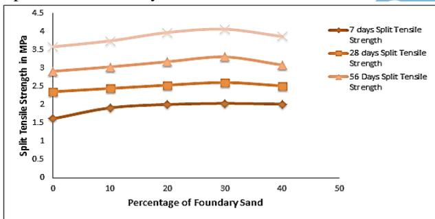
Figure-07. Split Tensile Strength and Percentage of Foundry Sand [4]
