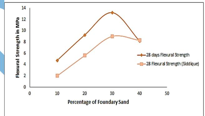
Figure-05. Percentage Variation of Flexural Strength for different foundry sand contents [3]
