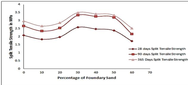
Figure-06. Split Tensile Strength and Percentage of Foundry Sand [3]
