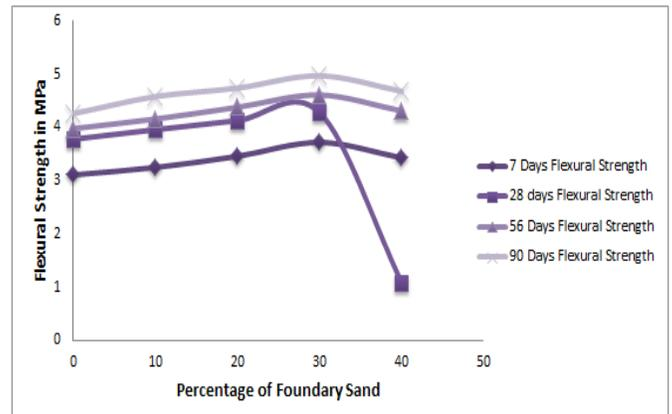
Figure-04. Flexural Strength and Percentage of Foundry Sand [4]
