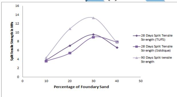
Figure-08. Percentage Variation of Split Tensile Strength for different foundry sand contents [3]
