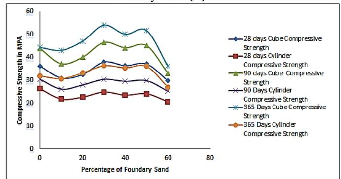
There is increase in compressive strength of cubes and cylinder at 25 to 30% replacement of foundry sand with fine aggregate, after 30% replacement the compressive strength of cubes and cylinder is start decreasing. As the duration increases the compressive strength is increasing. The highest compressive strength is observed at 30% replacement at 28 days and it is up to 50 to 55 Mpa [3].
