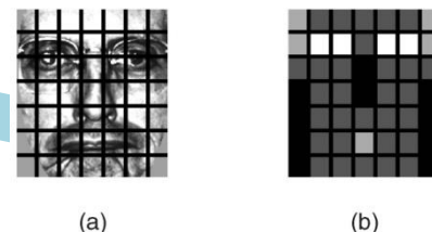
Fig.4. (a) A facial image divided into 7x7 windows. (b) The weights set for the weighted x^2 dissimilarity measure. Black squares indicate weight 0.0, dark gray 1.0, light gray 2.0, and white 4.0
