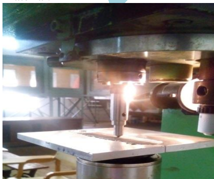
Fig: 15, Diamond cone impression on weld zone of FSW sample.
