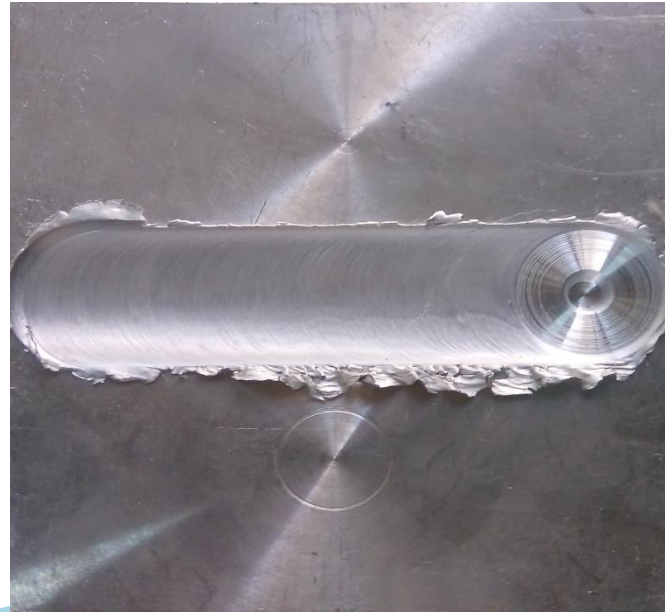
Fig: 14, Friction stir welded plates.
