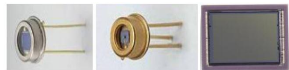
(a) Pin photo diode (b) Avalanche photodiode (c) Image sensor
