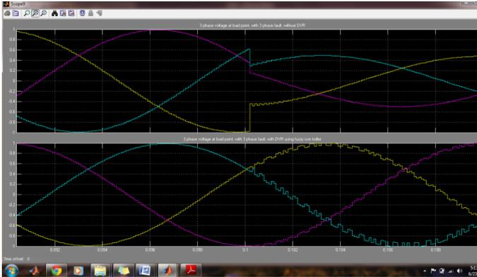
Figure 5.2; distortions in the PI compensated waveform
