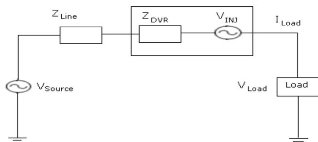
Fig. 3.2 Equivalent Circuit Diagram of DVR.
