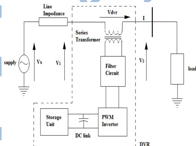
Fig. 3.1 Schematic Diagram of DVR
