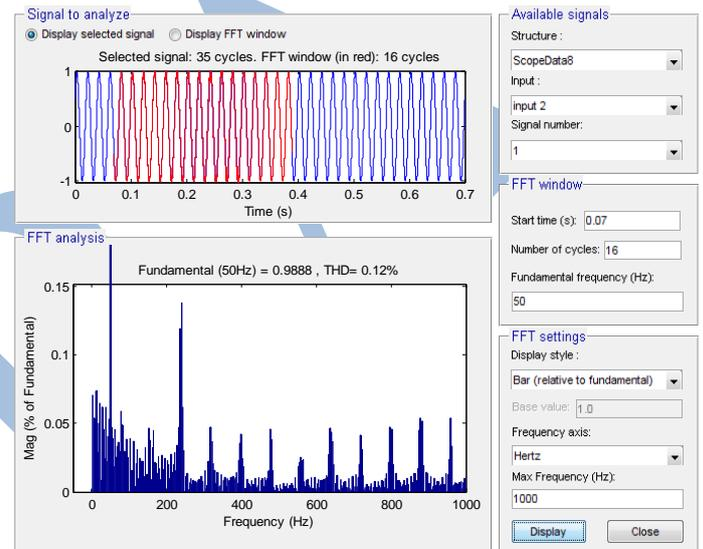
Figure 5.10: THD in case of BFO fuzzy controlled=0.12%
