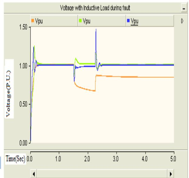
Fig. 3. Voltage characteristics graphs during voltage collapse
