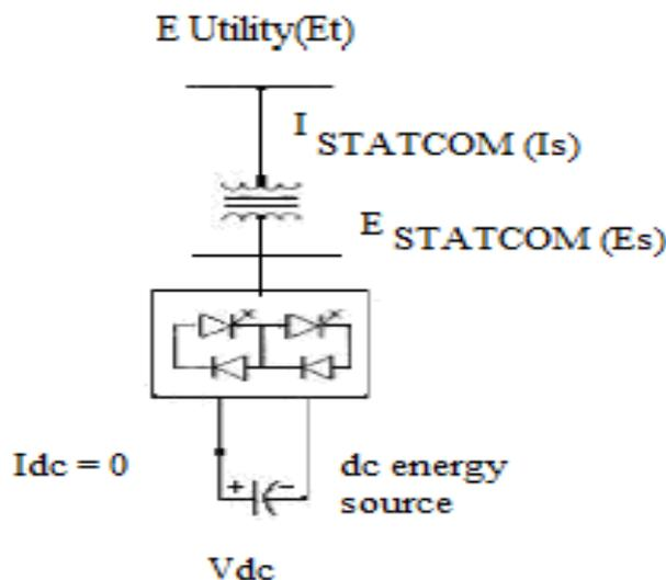
Fig. 2. A single-line STATCOM power circuit
