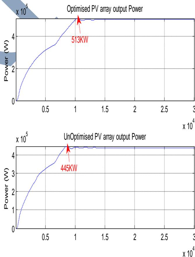
Figure 5.5: Comparison of Optimized and unoptimised power
