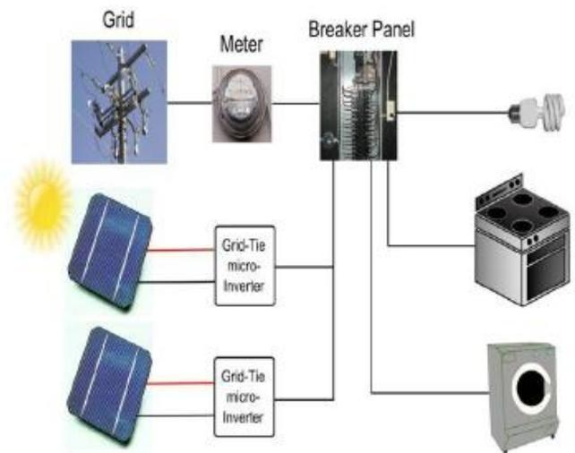
Fig 1.1: Schematic diagram of a simple photovoltaic system
