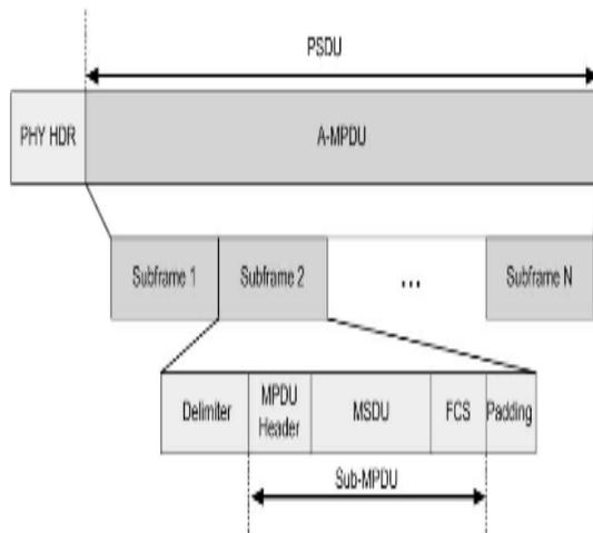
Figure 2: Frame Format of A-MPDU
