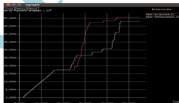
Fig-5 Showing Bit error rate in mode 3 and mode 2. The Bit error rate in mode 3 is less than in mode 2.
