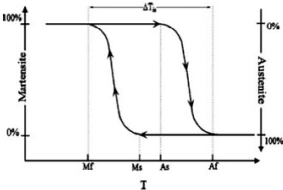
Fig.2. Stress- free martensite phase transformation.
