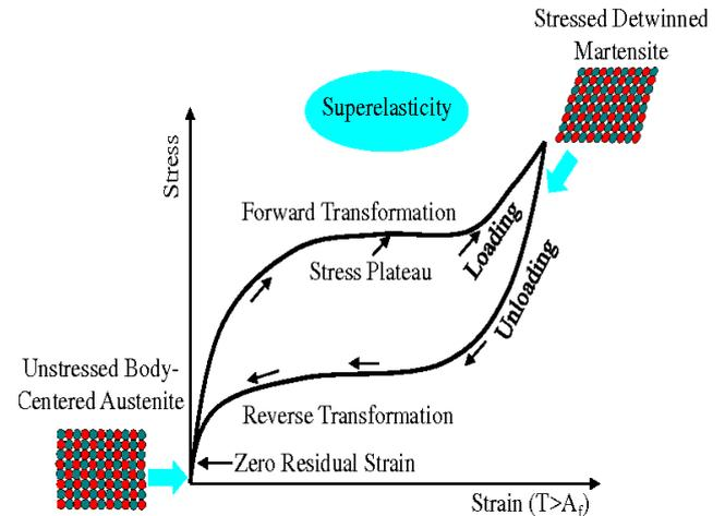
Fig.3 Isothermal stress induced martensite phase transformation
