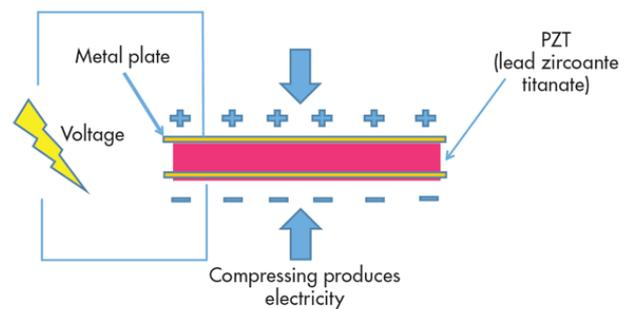
Fig.4. Piezoelectric effect
