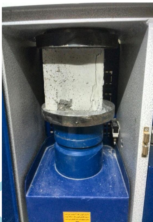
Figure 5. The Sample is Tested for Compressive Strength
