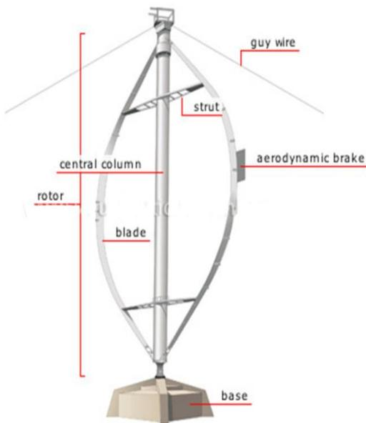
Fig. 1 Labeled parts of a Vertical wind turbine
