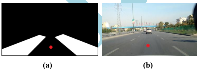
Fig. 6 (a) Base point on the mask image, (b) Base point on the road image.
