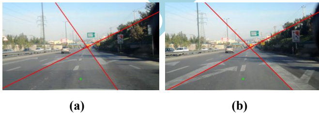
Fig. 9 (a) Incorrect detection of lane departure due to arrow markings on the road far from the camera, (b) Incorrect detection of lane departure due to arrow markings on the road near to the camera.
